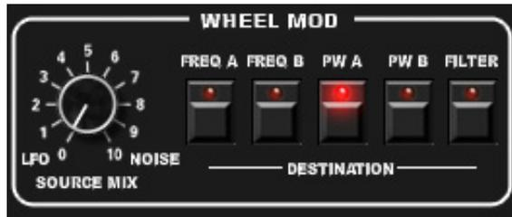
**Source Mix:** As an additional modulation signal white noise can be added.
