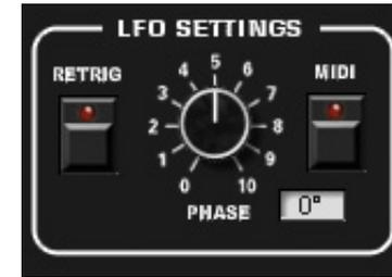
**Retrig:** Select between *Retrig* and *Free Run* modes. In the Free Run mode, the LFO runs continuously. In Restart mode, the LFO resyncs to the waveform phase position (restarted) whenever a key is struck on the MIDI keyboard.
