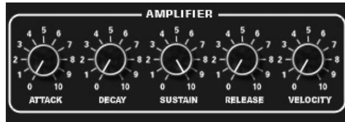
**Attack:** The duration of the first envelope segment. The volume level rises to its maximum value during the time adjusted here.
