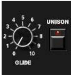
**Glide:** The time it takes for the pitch to glide from one note to the next. The Glide function does not have to be specifically activated – it is only necessary to enter a glide rate to enable it. Glide is off when the rate is 0.
